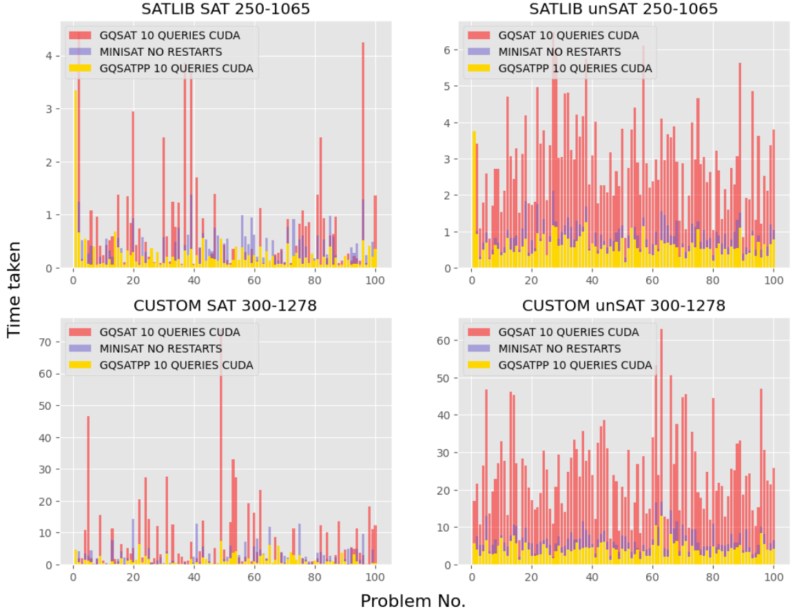
FIGURE 10. Time taken (in seconds) by selected algorithms to solve each of the problems in various testing datasets. The “10 QUERIES” suffix means that the graph neural network was queried for the first 10 branching decisions of the solution process for each problem (instead of the original 500). All solving algorithms were launched without restarts, since this way they yielded better results. For readability purposes, results for Graph-Q-SAT and Graph-Q-SAT++ with inference on CPU are not present since they are slightly worse than these for inference on CUDA.
