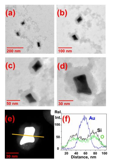
**Figure 3.** (**a**–**d**) TEM images of gold nanoparticles coated with silica using MPTMS. (**e**) STEM image of nanotag with an arrow indicating the EDX line scan position. (**f**) EDX line scan for Si K $\alpha$ , O K $\alpha$ , and Au L $\alpha$  signals of the particle shown in (**e**).
