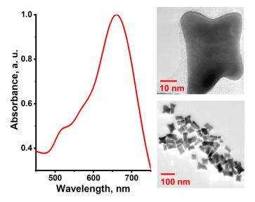
Figure 2. UV-Vis absorption spectrum and TEM images of bone-shaped gold nanoparticles.
