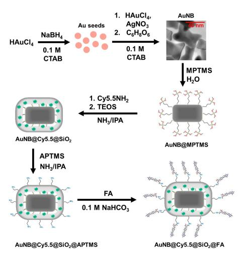
**Figure 1.** Scheme of the nanotags preparation including a synthesis of anisotropic gold nanoparticles, their labeling with a fluorophore, coating with a silica shell, and modification with a delivery vector.
