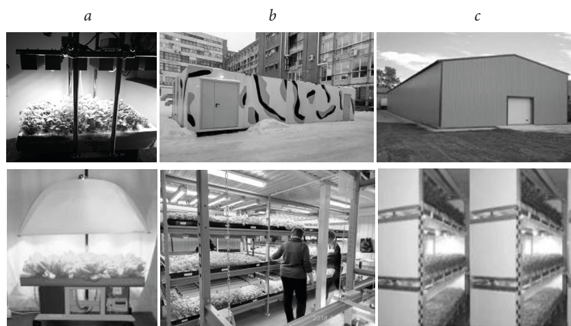
Fig. 1. Phytotechcomplexes developed at ARI, with controlled microclimate conditions and vegetation and lighting equipment based on resource-saving technologies for the high-quality plant production: (a) small-sized built-in, (b) mobile, (c) stationary
