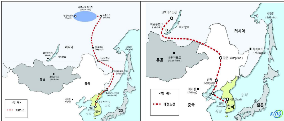
Figure 6 Russia-South Korea connecting gas pipeline route scenario
