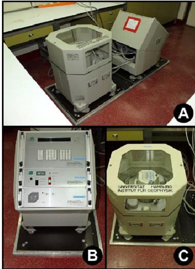
Figure 7: A) The ship-mounted gravimetric system. B) The gravimeter control unit. C) The gravimeter.
